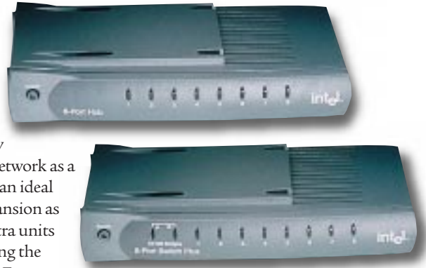
▲ LEDs ON THE FRONT OF HUBS, SUCH AS THESE INTEL MODELS, INDICATE THE STATE OF NETWORK ACTIVITY
